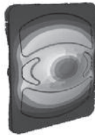
Prediction, optimization and testing of natural frequencies of assemblies (reduction of washer side panel vibration)
